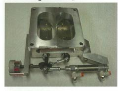
This Stop was designed to be used on TB1400 & TB1600 GET'M Garage Carbs with 2 oval blades and bore centerline of 2 1/4", oval bore is 2.200".
